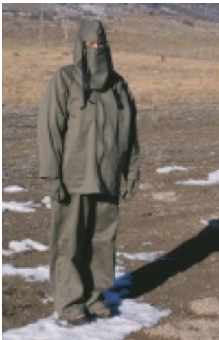
Subject wearing an odor-adsorbing suit. Subjects wore the jacket, pants, gloves, breath mask, and hood.
